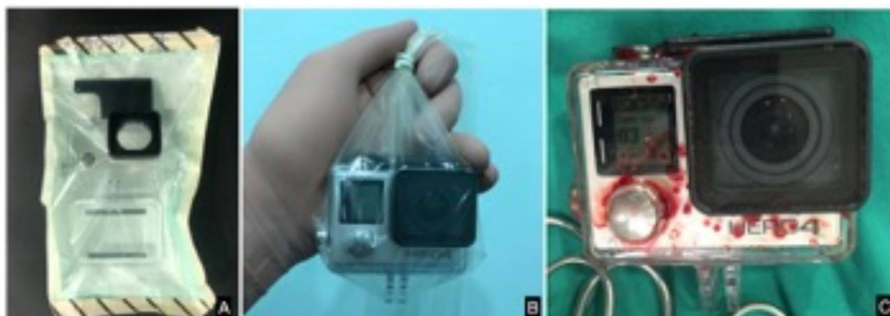
Fig. 1 (A) GoPro Camera Case Sterilized in Ethylene Oxide; (B) GoPro inside sterile ultrasound cover; (C) GoPro Camera in sterilized case, soiled after use
